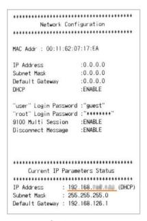
You can find the IP address of your printer under the "Current IP Parameters Status" section (underlined by orange above).
