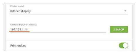
If automatic discovery fails, you can manually enter the IP address of the kitchen display device.
