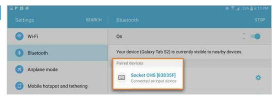
Tap on your Socket scanner in the list of Devices. After a few seconds, the "Not Paired" status will change to "Connected" or "Paired" and the scanner Blue LED will start blinking every 3 seconds, confirming the connection.
