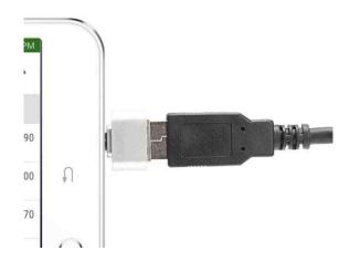
Then plug the the micro-USB end of the OTG adapter or cable into the micro-USB port of your mobile device and wait for the system to recognize the scanner.
