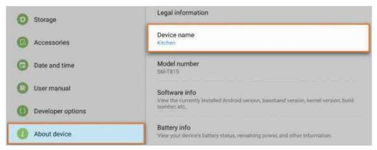
To configure a device name on an Android tablet, go to Settings > About device. On the next screen, tap Device Name, rename your device and tap OK.
